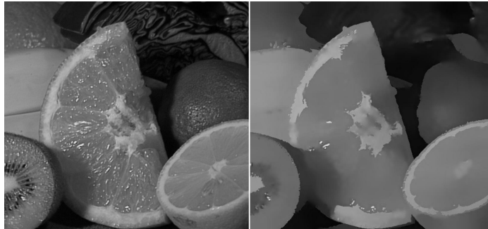
Figure 6-25: Mean-shift segmentation over scale using cv::pyrMeanShiftFiltering() with parameters max_level=2 , spatialRadius=20 , and colorRadius=40 ; similar areas now have similar values and so can be treated as super pixels, which can speed up subsequent processing significantly
