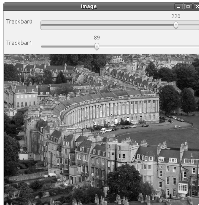
Figure 4-2: A simple application displaying an image; this window has two trackbars attached named "Trackbar0" and "Trackbar1"
