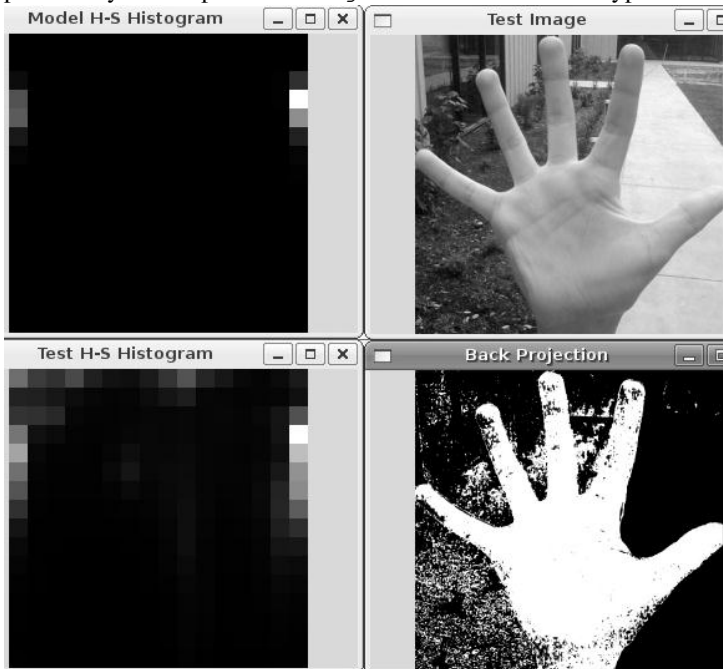
Figure 7-7, we use a flesh-color histogram to derive a probability of flesh image.
