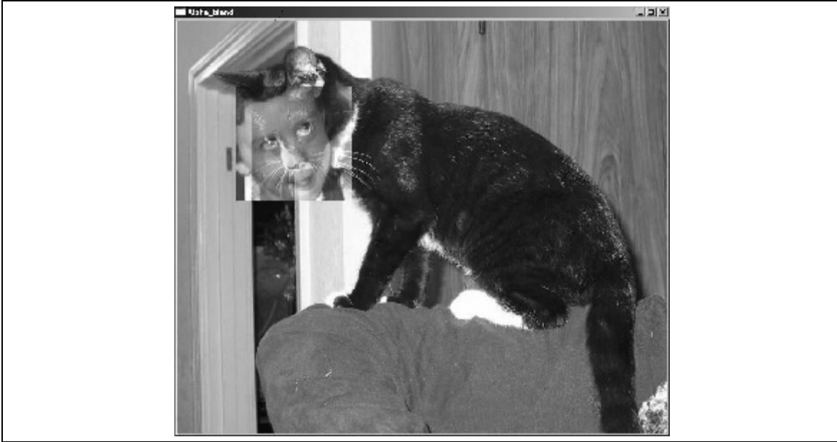
Figure 3-1: The face of a child is alpha blended onto the face of a cat
