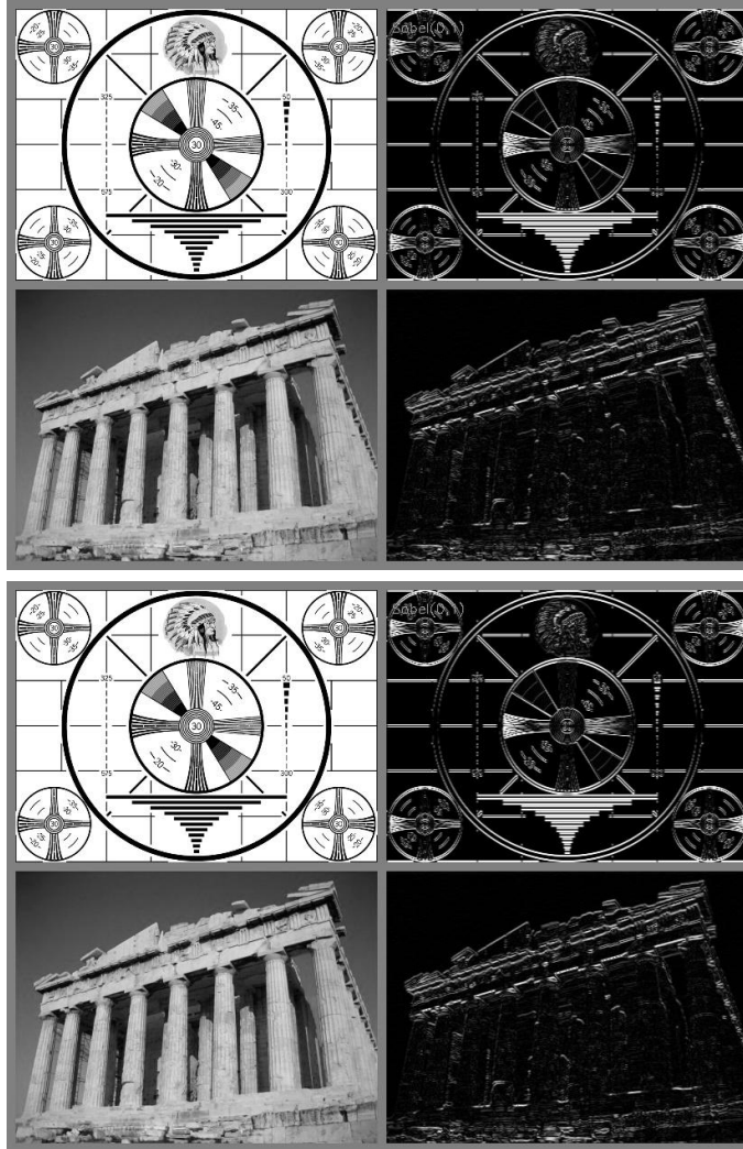
Figure 5-14: The effect of the Sobel operator when used to approximate a first derivative in the y -dimension.
