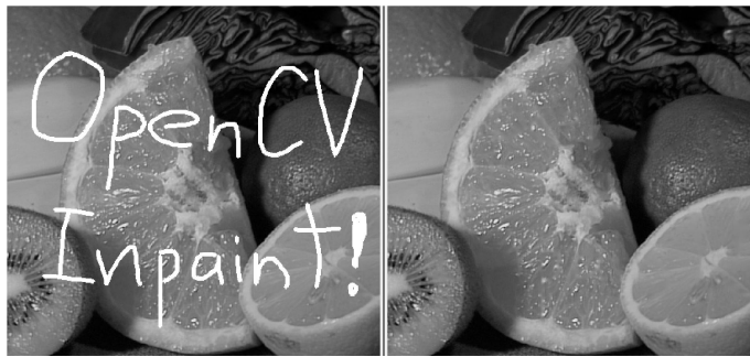
Figure 6-26: Inpainting: an image damaged by overwritten text (left) is restored by inpainting (right)
