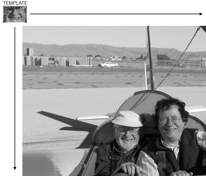
Figure 7-8: cv::matchTemplate() sweeps a template image patch across another image looking for matches
