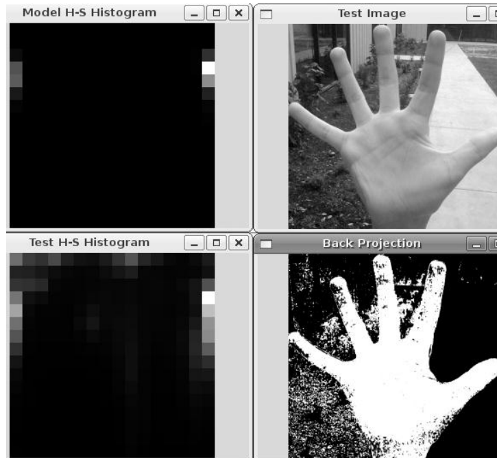
Figure 7-7: Back projection of histogram values onto each pixel based on its color: the HS (Hue and Saturation planes of an HSV representation of the image) flesh-color histogram (upper-left) is used to convert the hand image (upper-right) into the flesh-color probability image (lower-right); the lower-left panel is the histogram of the hand image
